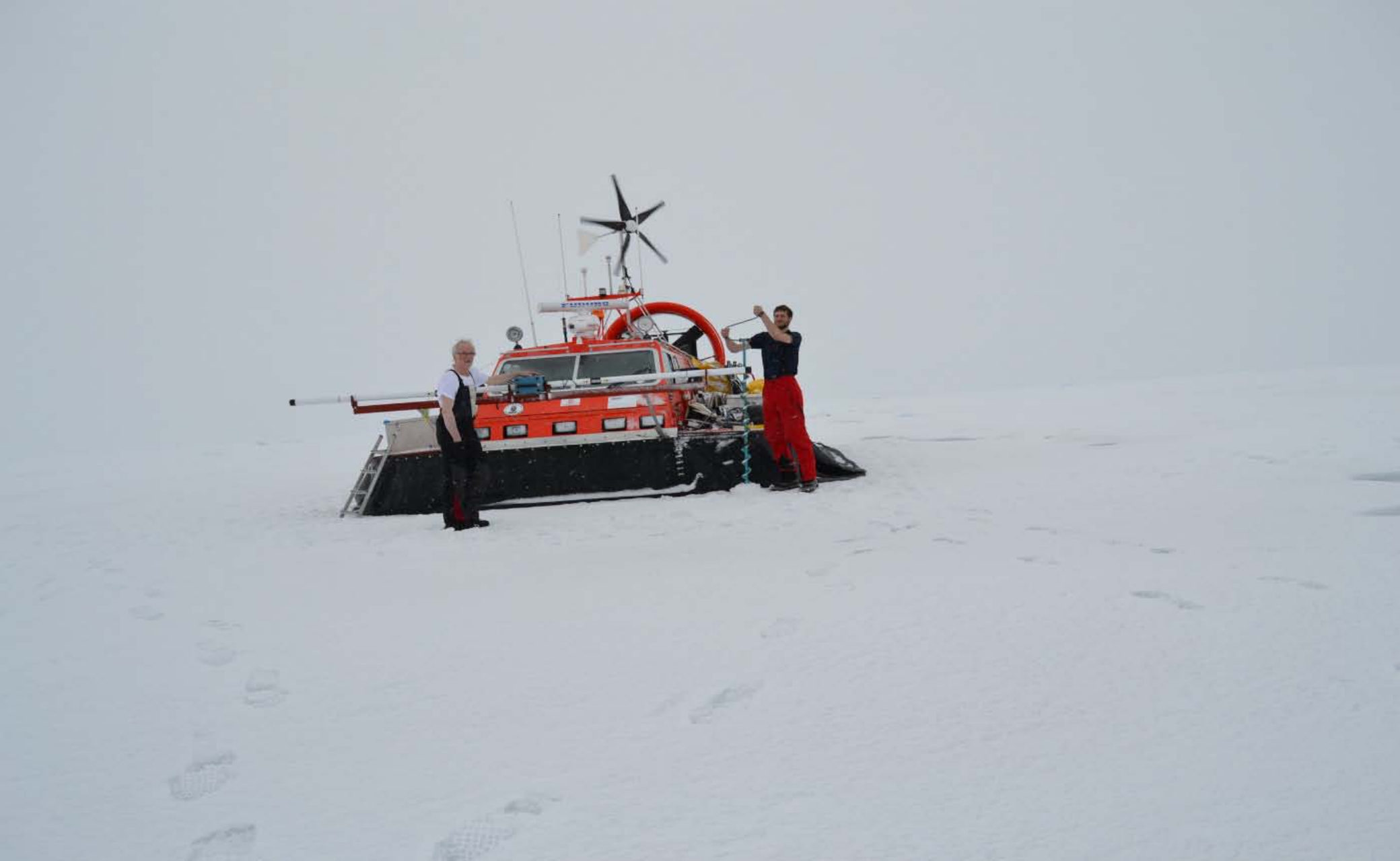
Calibrating the EM31 thickness measurements by augering a hole and making a direct measurement - Note the near white-out conditions with no horizon or shadows.
