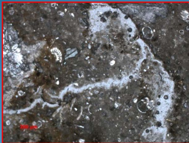
diapir D1 – authigenic dolomite with oxyhydroxides coating, serpulids traces
