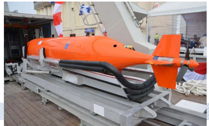
HUGIN AUV on back deck of KRI RIGEL
