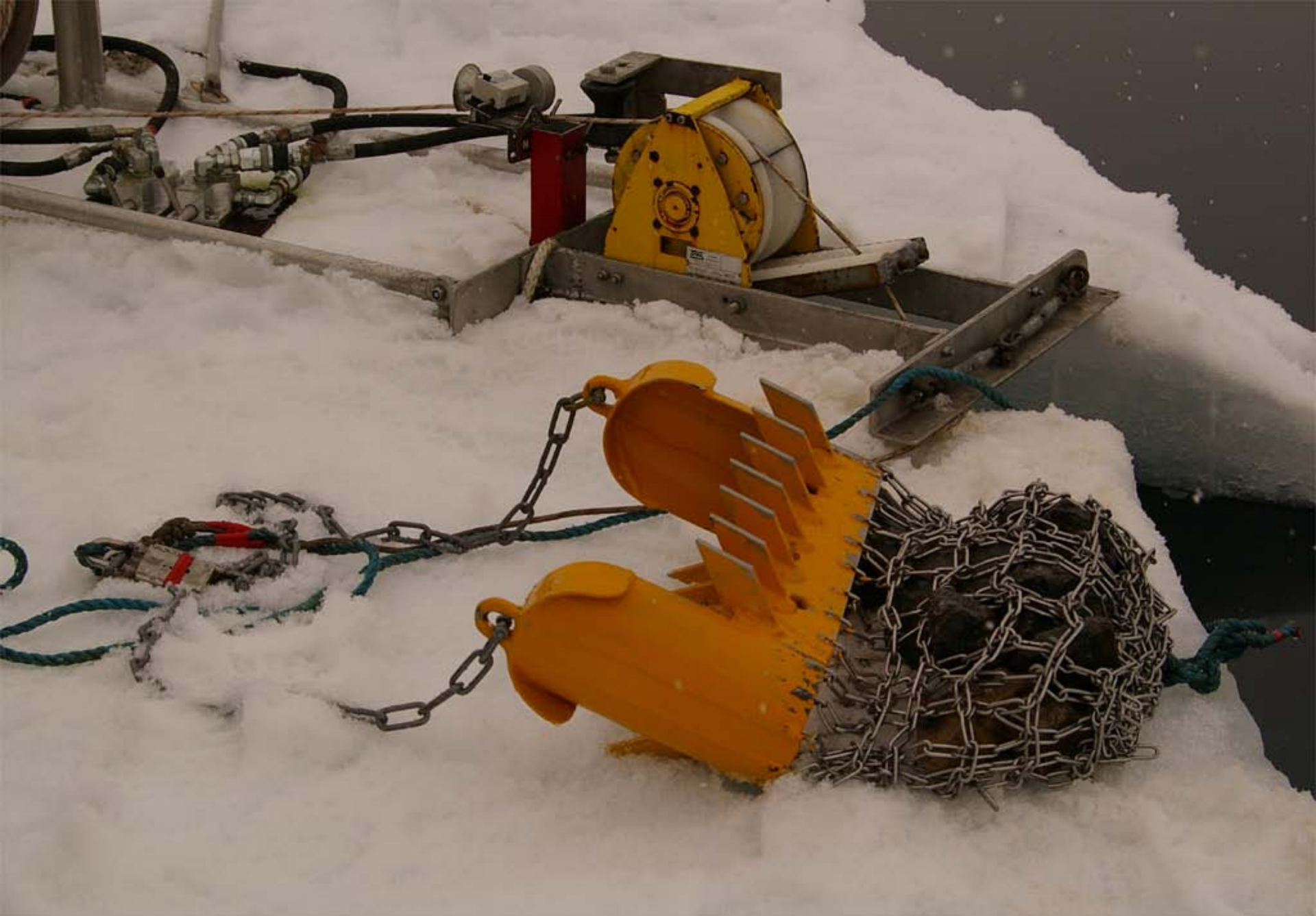
The Hydraulic Winch with Capstan Drive - three turns of kevlar aramid fiber rope
