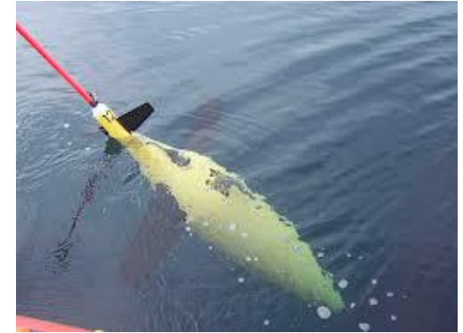
Christian Michaelsen Research (CMR) SailBuoy launched and recovered in the open sea
