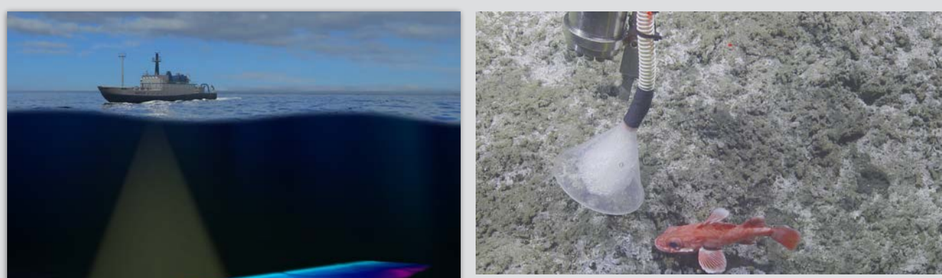
Figure 3 (above): ROV Hercules gathers seep bubbles with a funnel to collect in a gas tight chamber for gas composition analysis.
