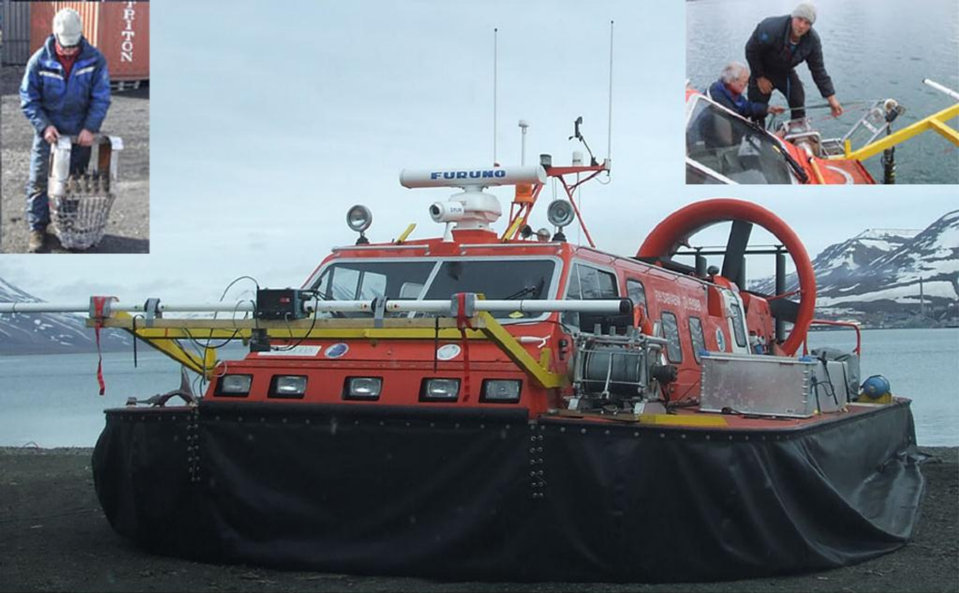
June 2009 Additions to the R/H Sabvabaa: Andreaa Seaguard AACP; rugged stainless steel dredge; Geonics EM-31 electromagnetic ice thickness measurements; Sea Bird SBE 19plus v2 CTD and 500 m single conductor cable on hydraulic winch.
