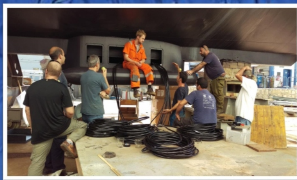
The Gondola before installation (left), and shown (right) below keel during installation of transducers.
