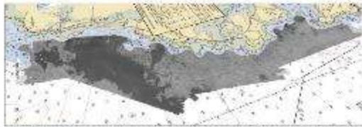
Bathymetric mosaic (2.5 m resolution) draped over the bathymetry surface (2.5 m resolution, 30 lines width, image visible). NOAA NED 15,000 used as a background. Resolution of image: 100m x 100m.
