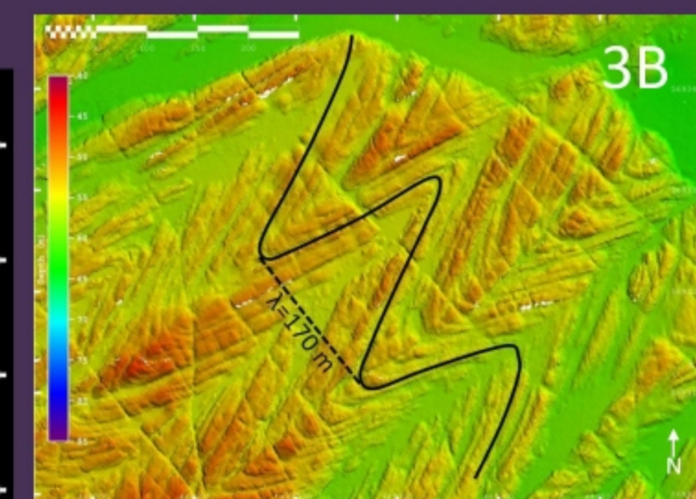
FIGURE 3B (above): Second order folding as indicated by wavelength ( \lambda ) measurement.
