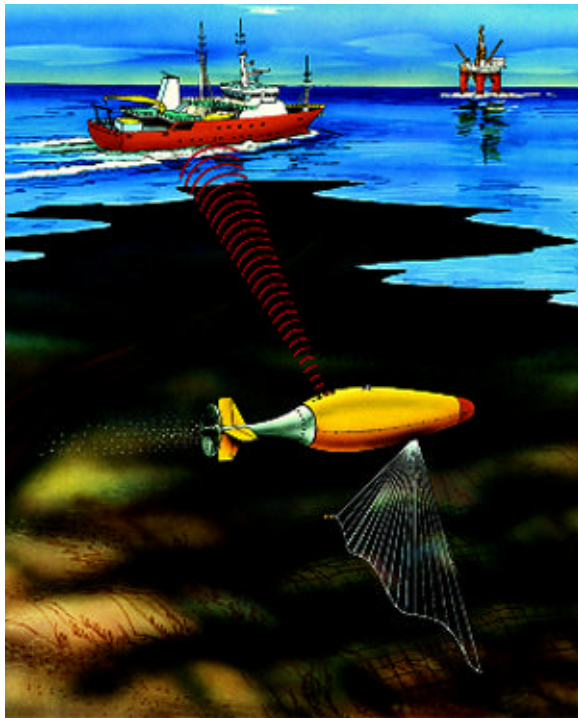
Figure 9: Left - The HUGIN AUV deploying a 200 kHz multibeam sonar (Figure courtesy of C&C Technologies). Transmission and visualization of data in real-time (above).
