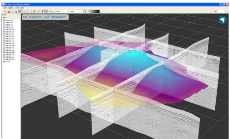
DELPH Seismic creates georeferenced vertical view of the subbottom profiles and models the picked horizons to build geoTIFF maps that can be exported to KMZ layers
