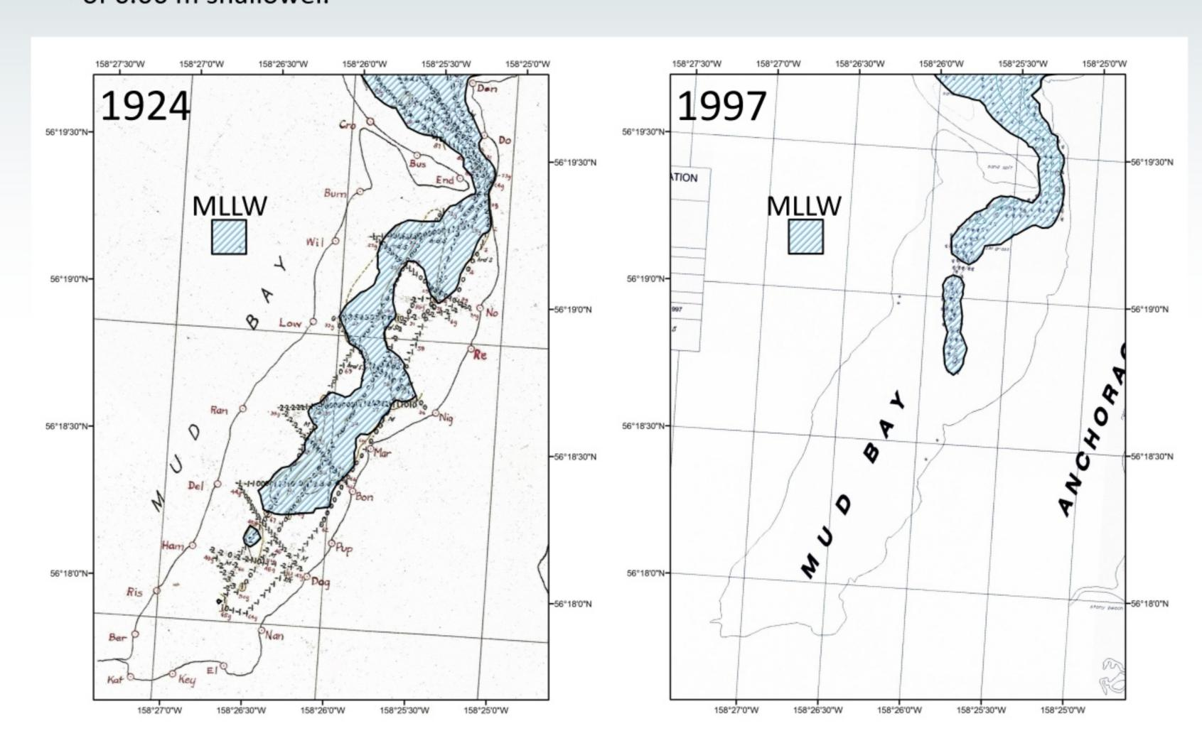
**Chignik Lagoon** lost 23.1% of its area at MLLW, and lost 16.3% of its volume when measured between MLLW and the deepest depths. This infilled area is an average of 1.27 m shallower.
