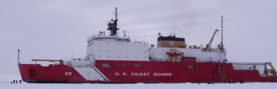
Length, Overall=128 metersBeam = 25 mPropulsDisplacement= 16,000 LTShaft HP = 30,000 HPProps =Cruising Speed= 12 knots.Max Speed - 17 kntsFuel CaIcebreaking = 1.4 m continuous, 2.44 m backing and rammingAccommodations = 19 Officer, 12 CPO, 54 enlisted, 35 (+15) scientist
