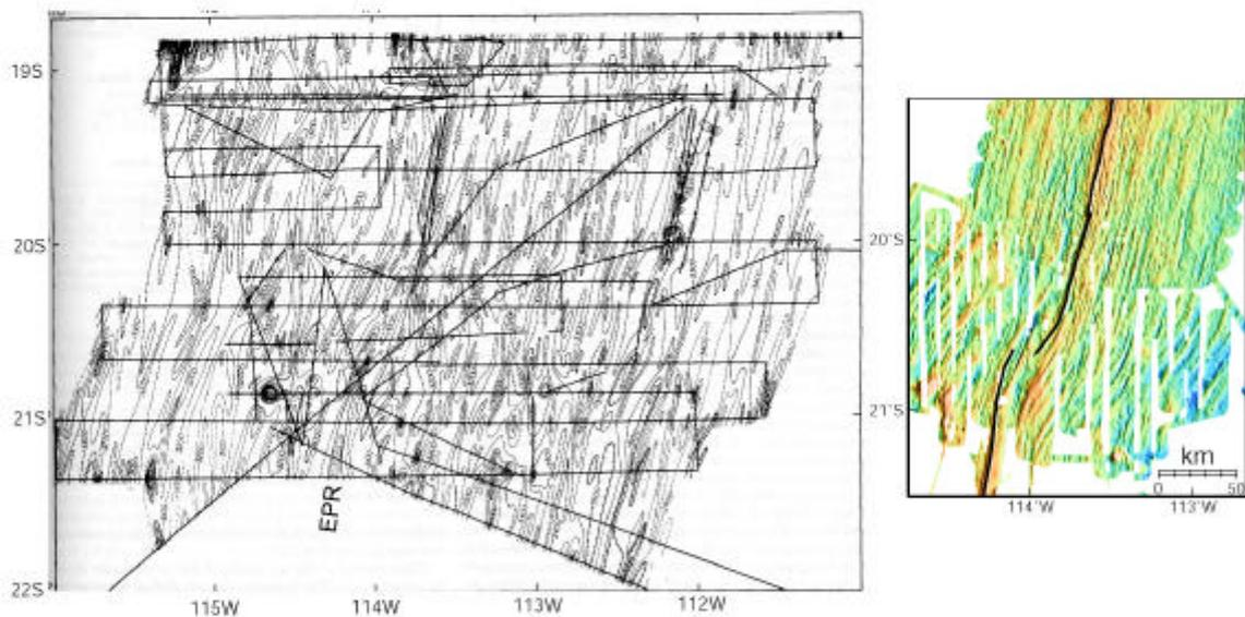
**Figure 2.** Comparison of conventional and multibeam bathymetry maps for the southern East Pacific Rise. (Left) A 30-km-wide non-transform offset was detected from conventional data [Rea, 1978]. (Right) Multibeam bathymetry shown at same scale reveals a large overlapping spreading centers (solid line). This discontinuity has slowly migrated southward, producing a 100-km-wide corridor of discordant seafloor fabric in its wake [Perram et al., 1993].
