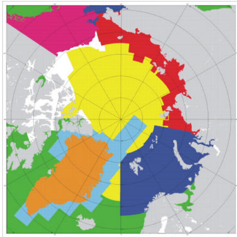
Figure 2. Segments of published maps and charts from which contour lines were digitised for the construction of the IBCAO grid.
