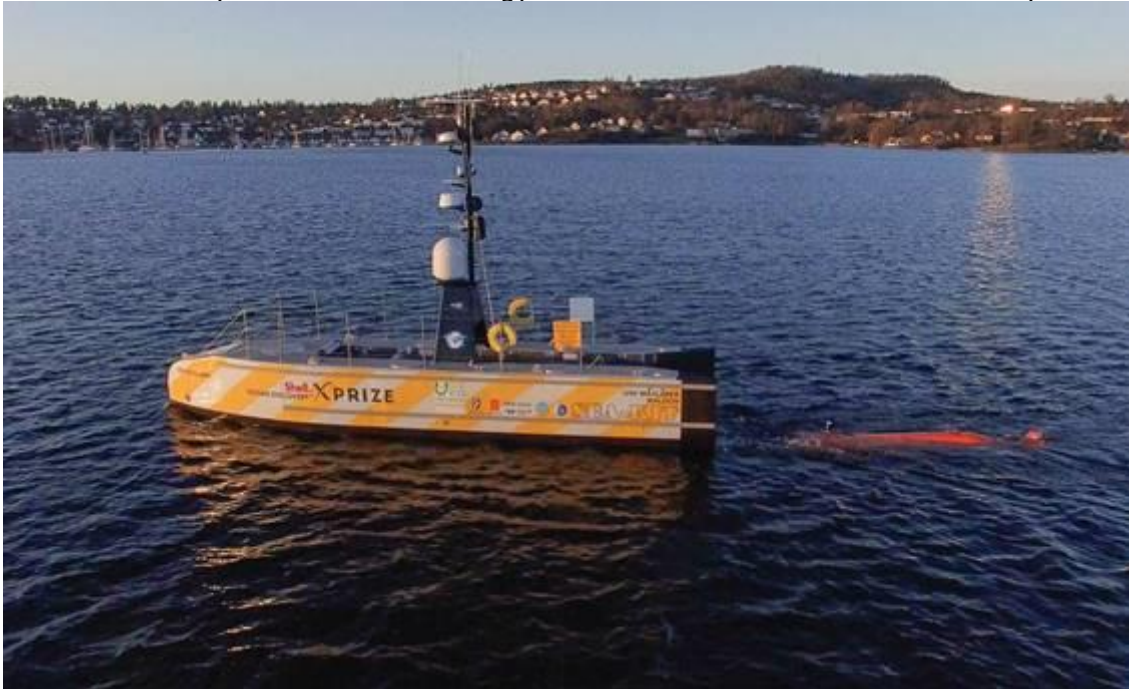
Drone footage capturing launch of the HUGIN AUV from the USV SEA-KIT (credit: Inner Space Center)
