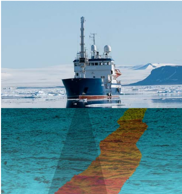
Bathymetry survey with multibeam echosounder
