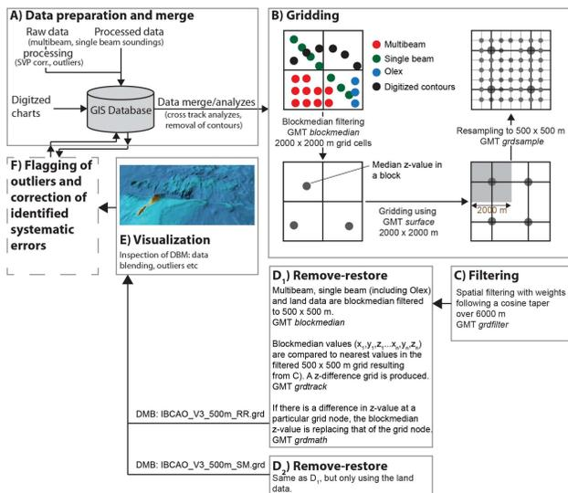
A Schematic illustration of the IBCAO compilation procedure. The main difference from the procedure used to compile IBCAO 2.0, is the final step consisting of adding multibeam, single beam (including Olex), and land data using the remove-restore method. Only single beam soundings with dense spatial coverage (close to or less than 500 m between soundings) are added in this final process, i.e. sparse random tracklines are omitted.
