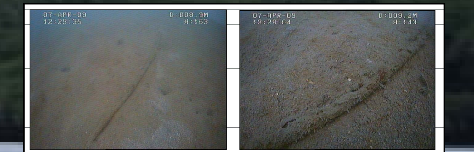
Remnants of metal cable protection in the eastern Southern Pipeline Route interpreted as the cause of the cluster of linear anomalies (above)
