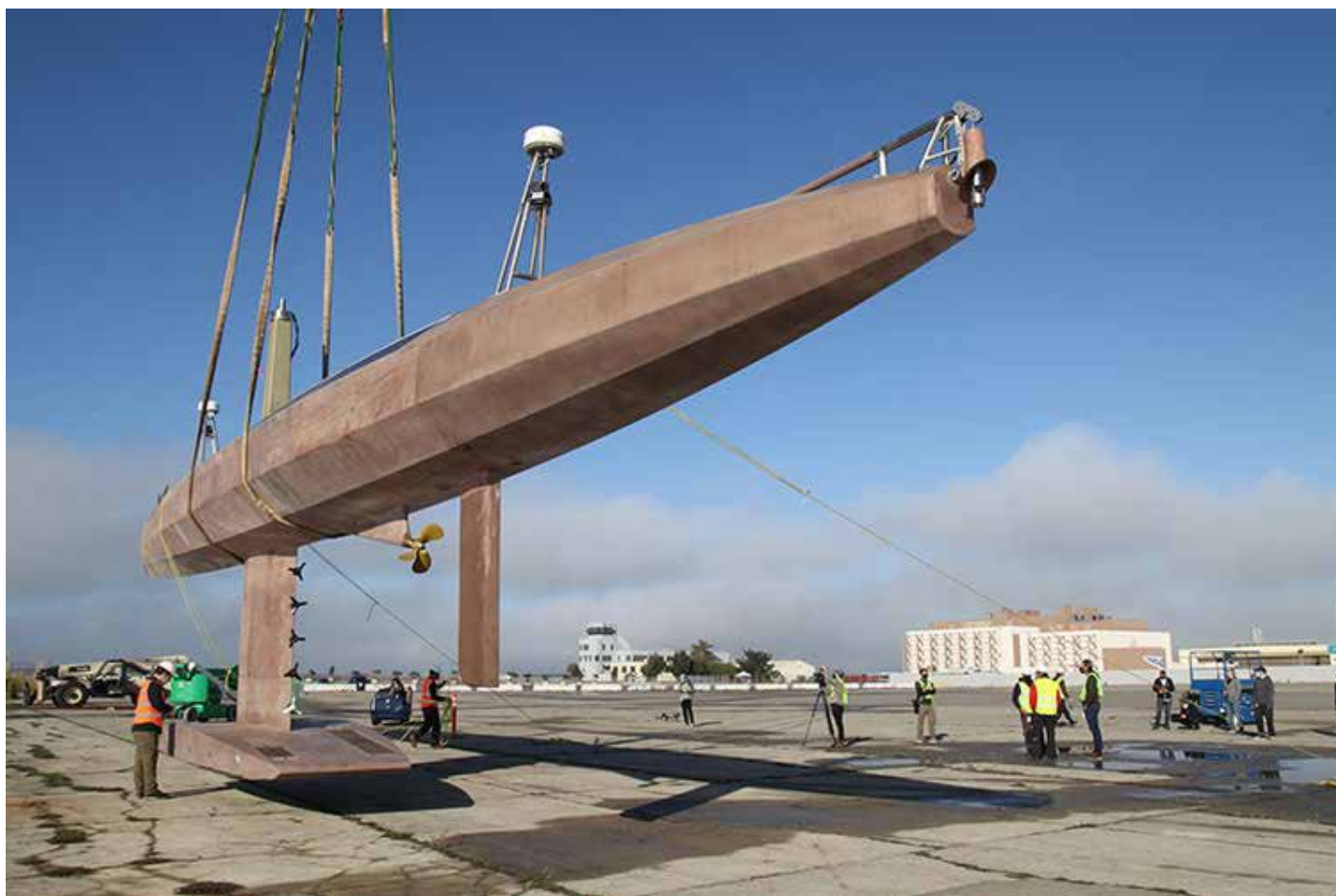
The Surveyor carries a sophisticated array of sonars in its keel, including the Kongsberg EM 2040 and EM 304, to map the seafloor to a depth of 23,000 feet (7,000 m). Credit: Saildrone
